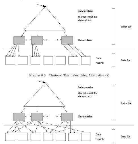
Figure 8.4 Unclustered Tree Index Using Alternative (2)
